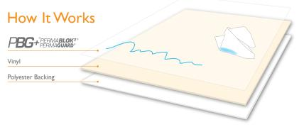
PBG+® acts as an invisible barrier against stains, allowing them to be cleaned off the surface with ease and virtually no harm to the vinyl.
